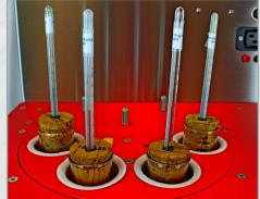
The SB+2 tests four (4) Cloud & Pour Point samples at a time. Accessories used with this Insert Module include Copper Sleeves, Glass Stators, Cork Rings & Discs, and Test Jar Stoppers.
