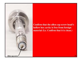
Confirm that the Allen cap screw that holds the Membrane Ferrule is torqued wrench-tight. The torque value should be 10 inch/lb. If the allen cap screw is only hand tight, not wrench tight to the appropriate torque value, the screw may protrude excessively. The extra Probe length may prematurely actuate the Foot Valve when the Probe is installed into the Housing.
