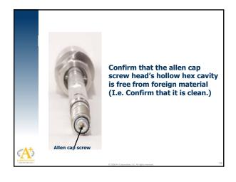
Confirm that the Allen cap screw that holds the Membrane Ferrule is torqued wrench-tight. The torque value should be 10 inch/lb. If the allen cap screw is only hand tight, not wrench tight to the appropriate torque value, the screw may protrude excessively. The extra Probe length may prematurely actuate the Foot Valve when the Probe is installed into the Housing.
