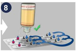
Carefully allow 4 drops of blue fluid to fall into each of the 6 circular wells on the test paddle ensuring that no sample is spilled into the viewing window
