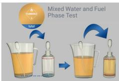
If there is visible free water but not enough to reach the 'Water line' when pipetted into the FUELSTAT® test bottle, continue pipetting fuel from near the bottom of the sample up to the top line marked 'Fuel line'
