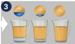
Agitate sample using a swirling motion and leave to **settle for 12-15 mins**. Once settled, is there any free water?
