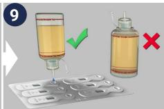
Keep the bottle inverted in case any additional drops may be required. If the bottle has been turned upright at any stage of this process it is important to return to step 5
