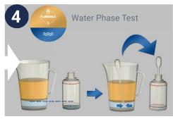
If enough free water in the sample, pipette water into the FUELSTAT® test bottle to the lower line, marked 'Water line'
