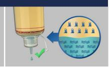
Only blue extraction fluid should be added to the test. If fuel is added to the test an incorrect result may be obtained (page 2 steps 6-8)
