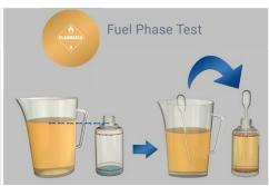
If there is no visible water in the sample, pipette fuel from near the bottom of the sample into the FUELSTAT® test bottle up to the top line marked 'Fuel line'
