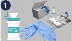
Clean sample equipment using 70% alcohol wipes and let dry. Have the FUELSTAT® test kit contents at hand. Wear Nitrile gloves when handling fuel.
